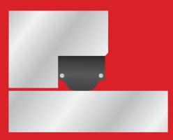
Cutaway of an S-seal designed for installation between the shaft of a piston and the barrel
