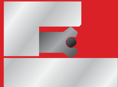
Cutaway of an O-ring energized seals
