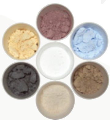
Glass, ceramic, stainless steel, carbon, various colors—just a sample of the varieties of filled PTFE that we offer.
